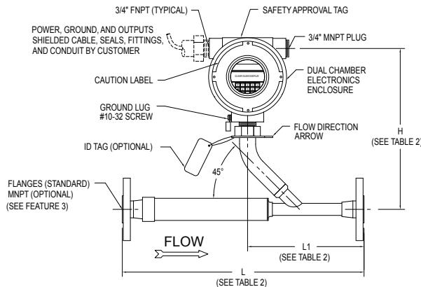
DIRECTLY ATTACHED ELECTRONICS ENCLOSURE (TA)
